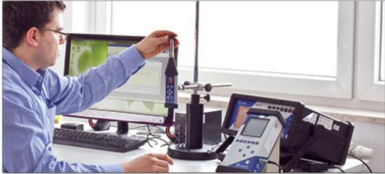
The SVAN 971 is a full class 1 instrument that has options for octave and third octave band filters. It has a measurement range of 15 dB to 140 dB which gives an incredible dynamic range that's greater than 110 dB. It can record audio comments to .wav files and measures both SLM (sound level meter) and dosimeter data.
